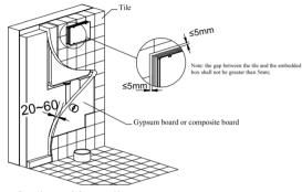
Cover the concealed systems with gypsum board or composite board and finally finish with tile paving. Wall paving thickness: minimum 20mm maximum 60mm;
